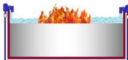
Figure 4.2 Schematic of Extinguishment by fixed system
