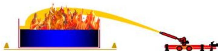
Figure 4.3 Schematic of Extinguishment by Mobile monitors
