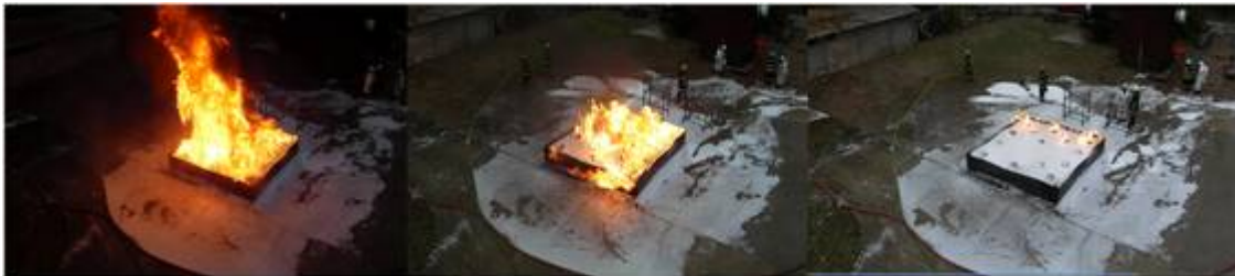
Figure 6.1 Photos from latest LASTFIRE bund fire testing
